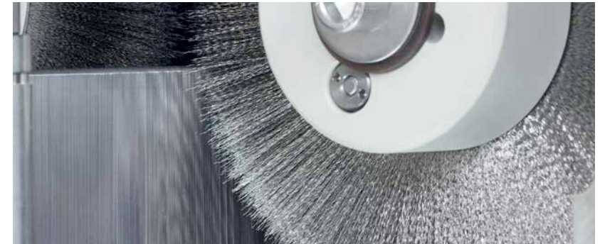
Cleaning drop wires
